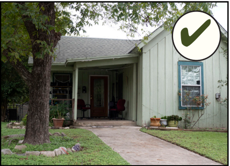
Board-and-batten siding is appropriate for the Historic District.
